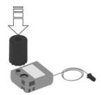
2. Turn the sealant bottle clockwise by 90° to the stop.
