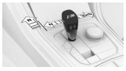
With the driver's seat belt fastened, press on the brake pedal and pull or push the selector
