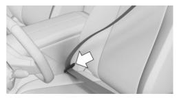
When the seat belt is fastened, the driver's and front passenger's belt straps are automatically tightened once after driving away.
