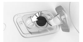
3. Place the fuel cap in the bracket attached to the fuel filler flap.
