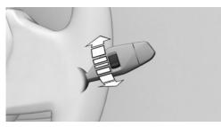
Turn the thumbwheel on the wiper lever.
