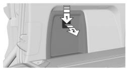
2. If necessary, remove the cargo cover from the storage under the cargo floor panel.
