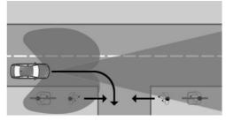
Sensors detect the traffic situation in their detection range when turning.
