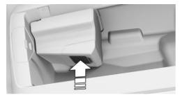
3. Remove the cover of the new fragrance cartridge. Hold the cover on the top to slide it from the fragrance cartridge.
