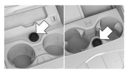
A socket is located between the cup holders in one of the marked positions. Detach the cover.
