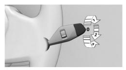
Turn the outer switch upward.
