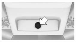
A socket is located in the center console. Detach the cover.
