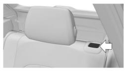
Pull the lever and fold the rear seat backrest forward.
