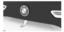
Press the button on the trunk to access the vehicle in deep sleep mode.
