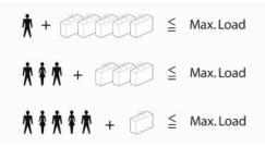
The maximum payload is the sum of the weight of the occupants and the cargo.
