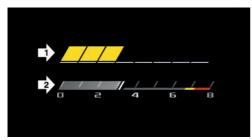
The shift lights, arrow 1, are displayed above the tachometer, arrow 2.
