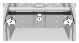
Pull out the cargo cover, arrow 1, and hook both sides onto the brackets, arrow 2.
