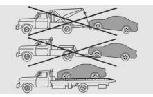
The vehicle should only be transported on a loading platform.
