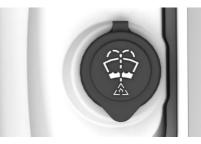
The washer fluid reservoir is located in the engine compartment.
