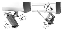
Insert the jack into the rectangular recess of the jacking point closest to the wheel to be changed.
