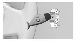
Turn the outer switch upward.
