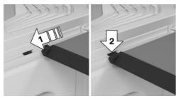
To restore the operability, close the cargo cover by hand, arrow 1, until it engages in the mounting, arrow 2.
