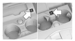
A USB port is located in the center console at one of the marked positions.
