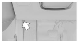
There is a diagnostic socket on the driver's side for reading out vehicle data.
